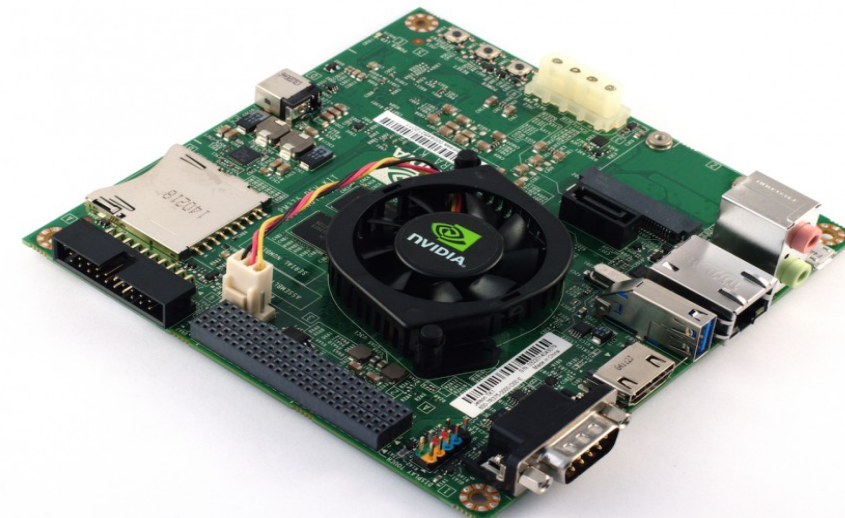
NVIDIA Jetson TK1 Devkit Kepler GPU with 192 CUDA cores 4-Plus-1 quad-core ARM Cortex A15 CPU
